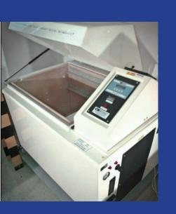
of weather. It can be used to determine the relative life of materials. The chamber is able to bring about changes in a few days or weeks that would naturally take months or years.
